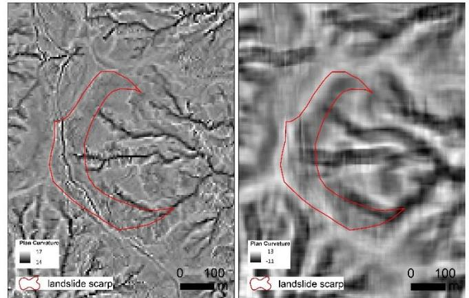
Figure 4. An example of a scaled predictor in relation to a landslide scarp. Left image: plan curvature at the default scale. Right image: plan curvature scaled in a 9×9 window. Note a north-south trench inside the landslide scarp on the left image that is filtered out on the right image.
